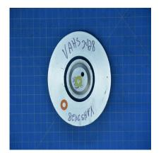
T103310-101 - FREEWHEEL ASSEMBLY REMOVAL SET, RENTAL TOOL, FOR USE ON BELL HELICOPTERS
