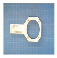
T103308-101 - FREEWHEEL ASSEMBLY CAP FIXTURE, RENTAL TOOL, FOR USE ON BELL HELICOPTERS
