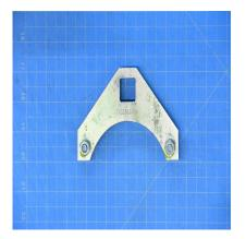
T103306-101 - INPUT ADAPTER SPANNER SET, RENTAL TOOL, FOR USE ON BELL HELICOPTERS
