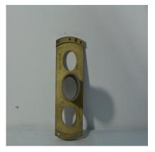
T103203-101 - COLLECTOR SHAFT HOLDING FIXTURE ASSEMBLY, RENTAL TOOL, FOR USE ON BELL HELICOPTERS
