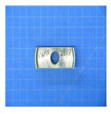
T103132 - TRANSMISSION BEARING PUSH BAR, RENTAL TOOL, FOR USE ON BELL HELICOPTERS
