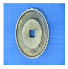
T103071 - MAIN TRANSMISSION LOWER COLLAR GEAR DUPLEX BEARING NUT WRENCH, RENTAL TOOL, FOR USE ON BELL HELICOPTERS
