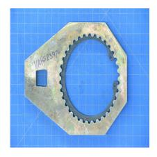
T103033 - TAIL ROTOR GEARBOX SLEEVE WRENCH, RENTAL TOOL, FOR USE ON BELL HELICOPTERS
