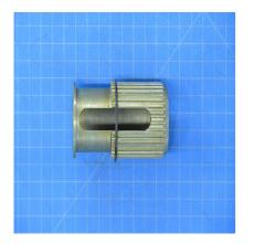
T103025 - MAST TORQUEMETER PLUG, RENTAL TOOL, FOR USE ON BELL HELICOPTERS
