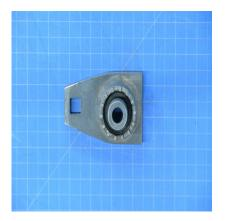
T103017 - SPLINED FREEWHEEL NUT WRENCH ASSEMBLY, RENTAL TOOL, FOR USE ON BELL HELICOPTERS
