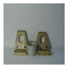
T102045 - MAIN ROTOR HUB GRIP SPACING TOOL, RENTAL TOOL, FOR USE ON BELL HELICOPTERS
