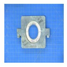
T101589 - BEARING REMOVAL PLATE, RENTAL TOOL, FOR USE ON BELL HELICOPTERS
