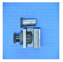
T101572 - PLANETARY BEARING FIXTURE, RENTAL TOOL, FOR USE ON BELL HELICOPTERS
