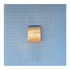
T101506 - PLANETARY SHAFT SLEEVE, RENTAL TOOL, FOR USE ON BELL HELICOPTERS
