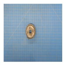
T101502 - GEARSHAFT NUT WRENCH, RENTAL TOOL, FOR USE ON BELL HELICOPTERS
