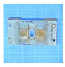
T101400 - MAIN ROTOR ADJUSTMENT SUPPORT, RENTAL TOOL, FOR USE ON BELL HELICOPTERS
