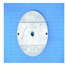
T101392 - SCISSORS AND SLEEVE ASSEMBLY WRENCH, RENTAL TOOL, FOR USE ON BELL HELICOPTERS
