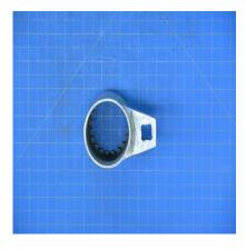
T101305 - INTERNAL SPLINE WRENCH ASSEMBLY, RENTAL TOOL, FOR USE ON BELL HELICOPTERS
