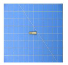
HL19PB6-7 - Rivet Pin, Cadmium, Alloy Steel, Flush Shear Head
