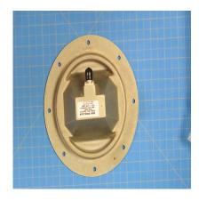
DMPN3-3/A - Antenna, Radar Altimeter
