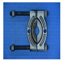
CJ951 - BEARING SEPARATOR, RENTAL TOOL, FOR USE ON BELL HELICOPTERS
