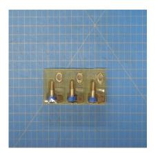
3852A-282-252A - Potenitiometer 2.5K Ohm 2W Variable Resistor
